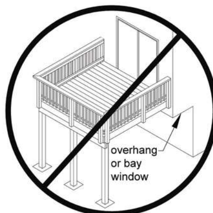
Figure 18: No Attachment to House Overhang
